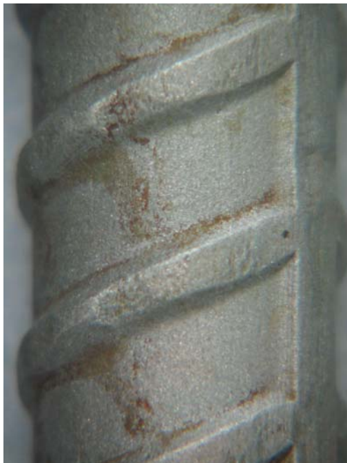
Sandblasted 2201: widespread superficial corrosion
