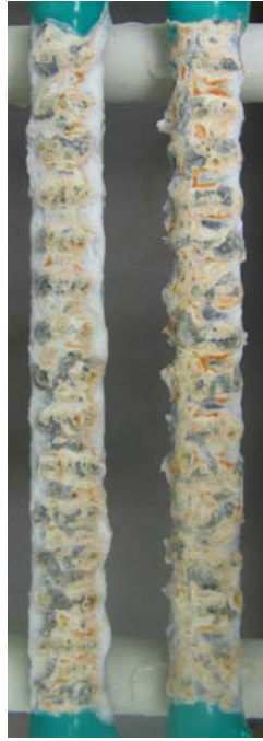
Galvanized-Type B-hole 3Cr12-sandblasted
