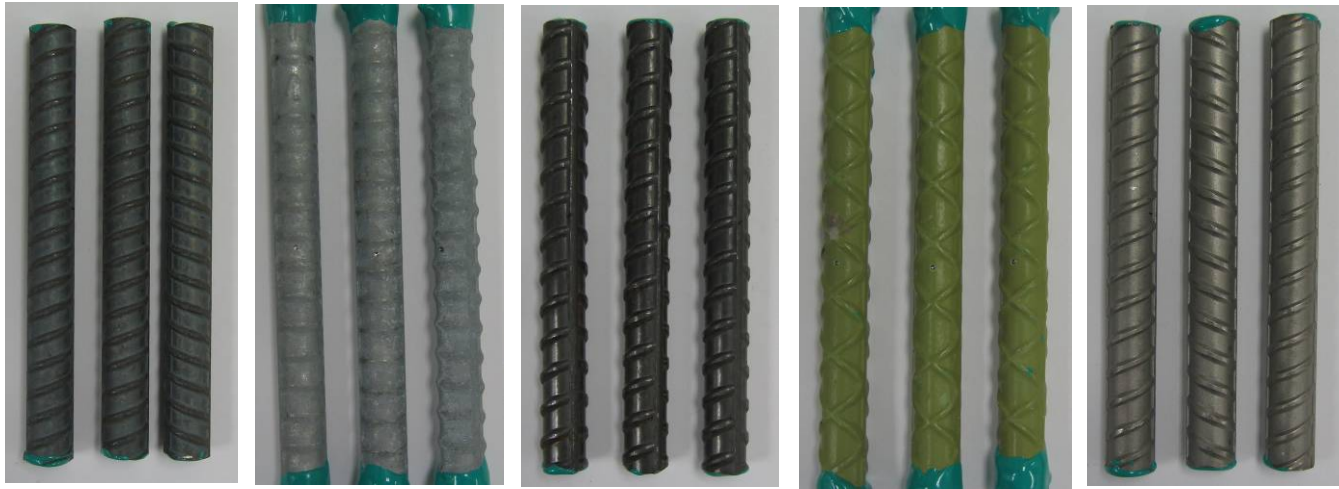
Figure 1. Condition of selected bars before exposure. From left to right: A615-as received; Galvanized-Type B-hole; A1035-as received; ECR-Type B-hole; and 2205-as received.
