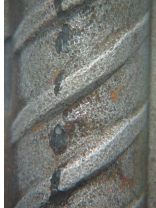
Sandblasted 3Cr12: extensive corrosion, pits and general
