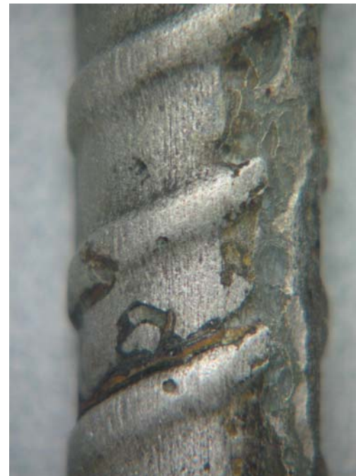
Sandblasted A1035: broader pitting attack
