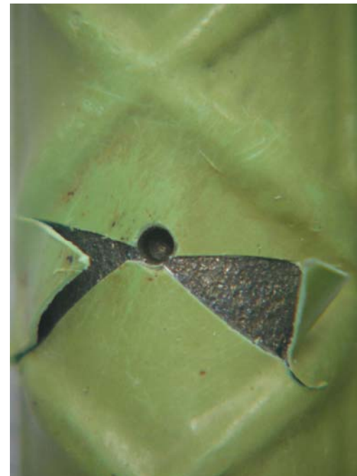
ECR-Type B- adhesion: coating easy to peel: rate-5
