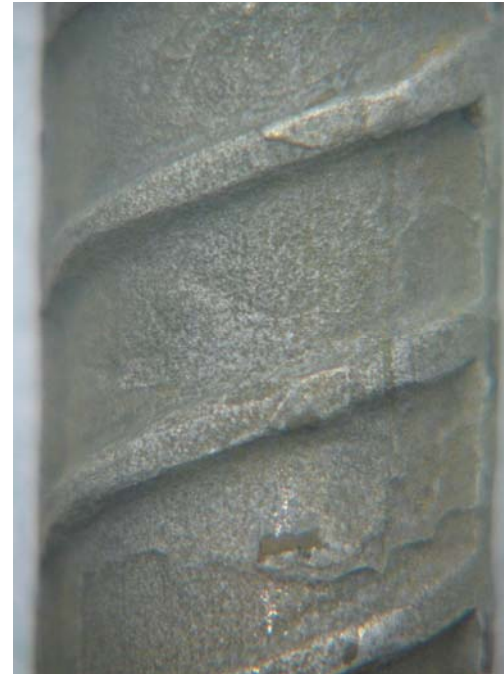
Sandblasted A615 bar: extensive corrosion, more uniform
